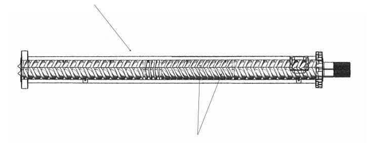
**TWIN SCREWS** – Twin counter rotating intermeshing screws act as a positive displacement pump when rotated. They compress and release the material several hundred times from beginning to end of each section.
